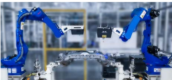
Subframe Inline Measurement
