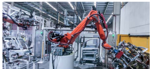
Vision-Guided Car Door Inner Panel Picking
